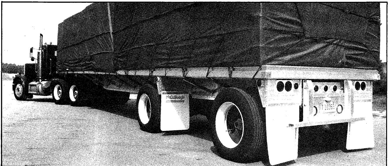
Loaded aluminum trailer ready to make delivery run with 4200 extra pounds of payload.
