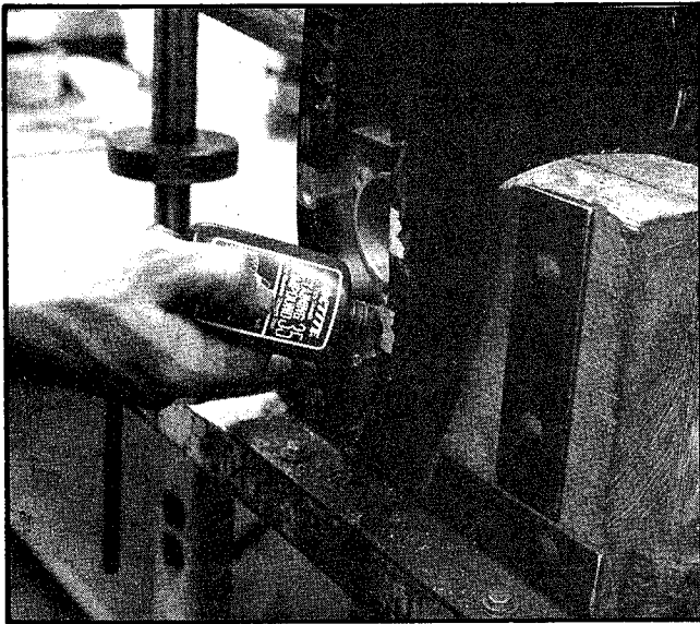
Steel studs are retained in aluminum lower end unit. Liquid is being inserted into blind hole.
