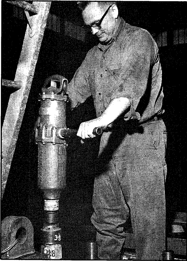
The old way of mounting giant studs. Jack hammers were used to force huge studs into castings. Some studs broke, some castings failed.
