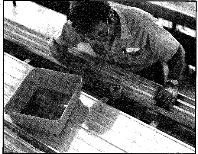
Flat bed parts are bonded together with Loctite structural adhesive.
