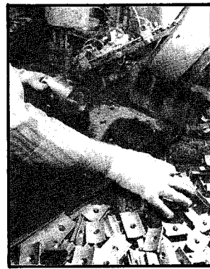
Four photos illustrate treatment of starter pole piece screws with threadlocking adhesive to prevent loosening.
