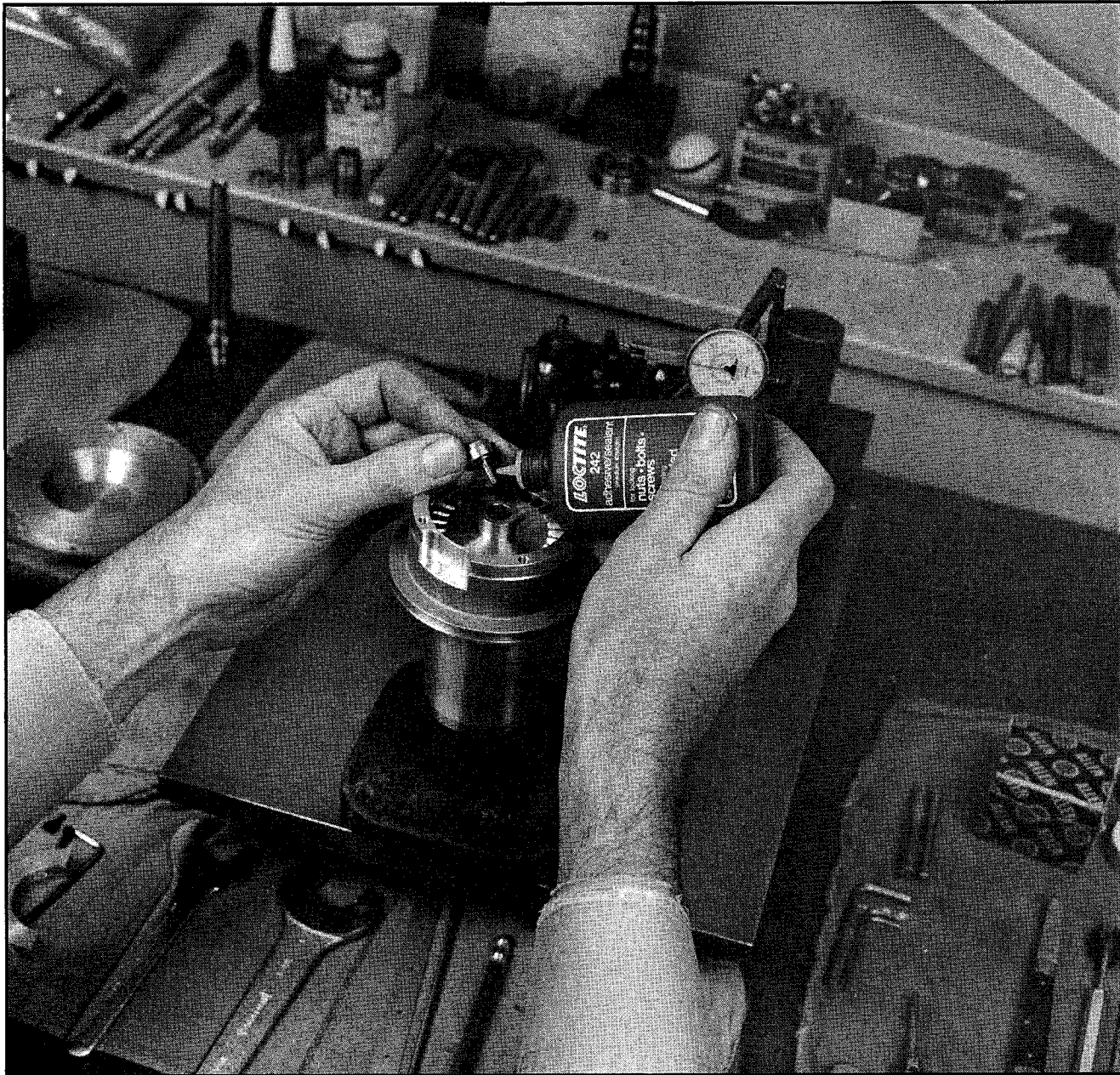
Threaded fastener in high speed spindle is secured with anaerobic threadlocker. Assembly spins at 30,000 RPM.
