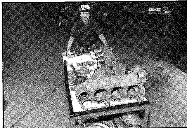
All engine parts for Continental engine are kept together throughout their life cycle. Rolling stand contains a complete engine.
