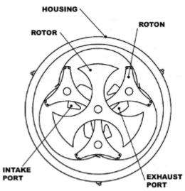
The **Legacy Engine** can best be described as a planetary rotary engine comprised of a central rotor and orbiting elements, named RoTons.
