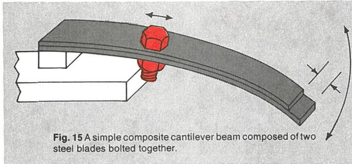
Fig. 15 A simple composite cantilever beam composed of two steel blades bolted together.
