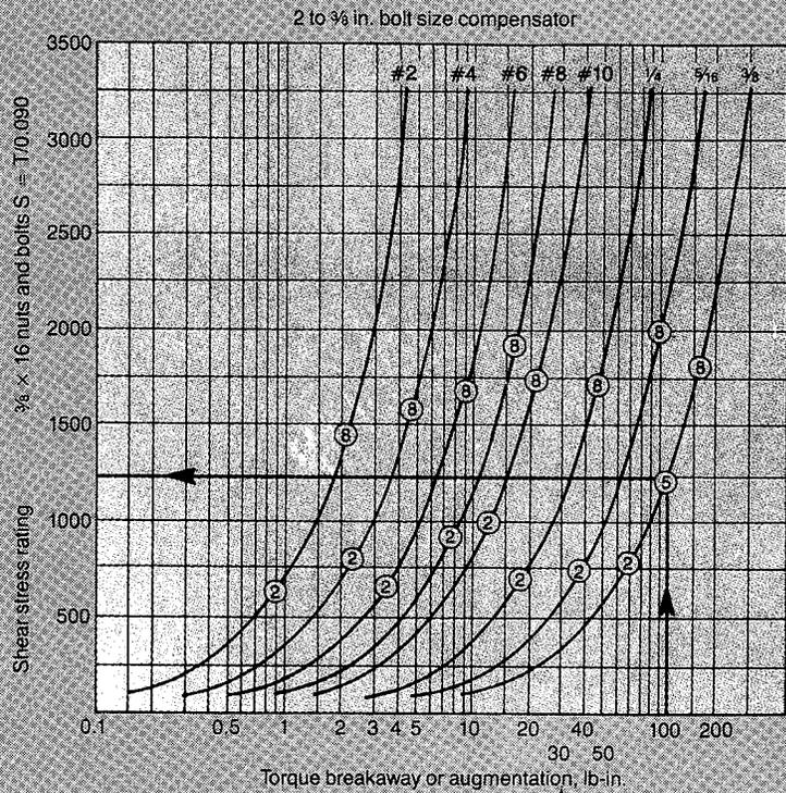
Example:  $\% \times 16$  G5 recommended torque is 360 lb-in., 30% is 108 lb-in. materials below the horizontal line are safe to use with standard nut.
