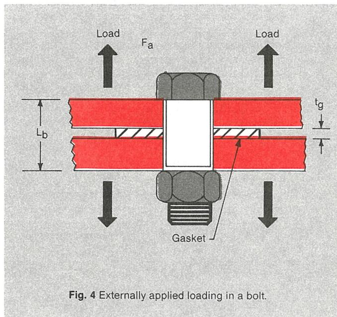
Fig. 4 Externally applied loading in a bolt.
