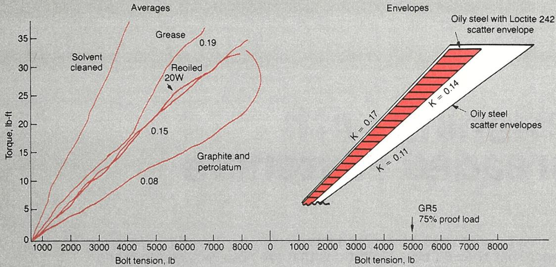
Fig. 1 Torque tension averages and envelopes grade 5 steel.
