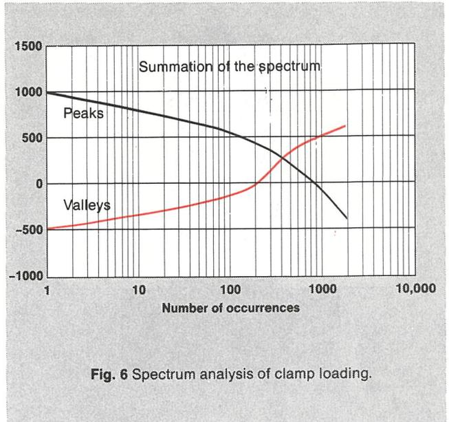
Fig. 6 Spectrum analysis of clamp loading.
