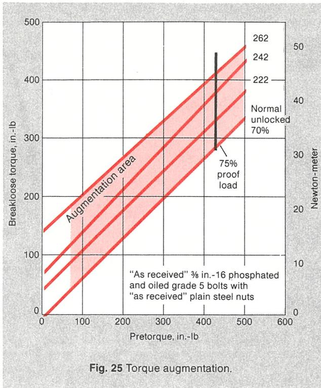
Fig. 25 Torque augmentation.
