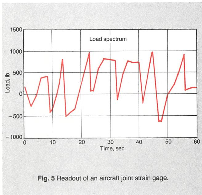
Fig. 5 Readout of an aircraft joint strain gage.
